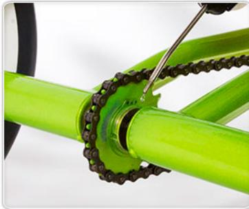
Place two drops of oil on the rear axle on either side of the toothed gear sprocket where the plastic chain guard rests to prevent squeaking.
