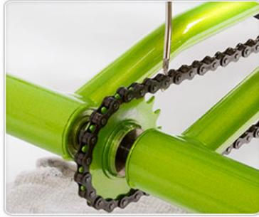
Apply a moderate amount of oil along the chain. Release the brake, and raise the left rear drive wheel off the ground and rotate the pedals to distribute the oil evenly.
