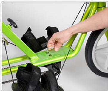
To tighten the chain, begin by loosening the two screw caps on top of the crankcase using the 3/16" hex-head wrench.
