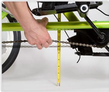
To check the chain tension, lift the lower chain. There should be no more than 1" of deflection. If the chain tension is fine, it is still a good idea to check the tightness of the 2 cap screws.
