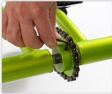
Tighten the rear sprocket screw with the 5/32" hex-head wrench. The gear sprocket should be centered left-to-right on the rear axle when tightened.
