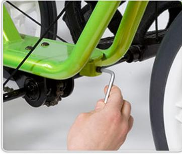
Use the 3/16" hex-head wrench to adjust the bolt screws at the front of the plate. This tightens the chain. When the chain tension is right, tighten the 2 cap screws on the top of the crankcase.
