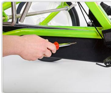
Use a Phillips screwdriver to remove the screw in the side of the chain guard.
