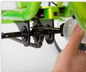
Place two drops of oil on either side of the front gear sprocket.
