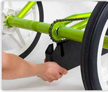
Detach the back of the bottom cover by pushing down.
